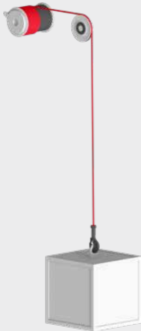
lifting of an unguided load on a single fall
